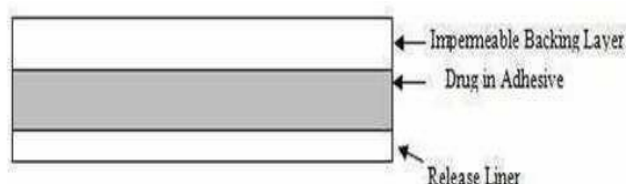
Fig. 1: Design of Drug Inadhesive Type Transdermal Patch
